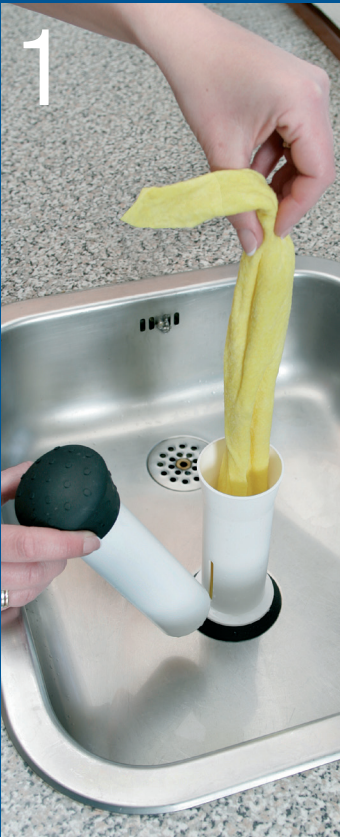
1 Remove the piston from the tube. Lower the wet cloth into the tube.
